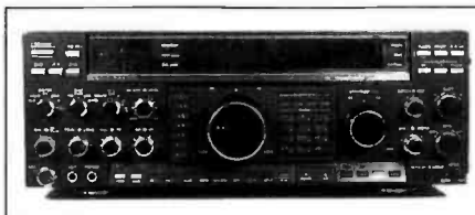
FT 1000 Is it the world's no.1 TCVR. Should be. 200w multimode. Rx-100k -30MHz DEPOSIT £1499 plus 9 x £199.99
