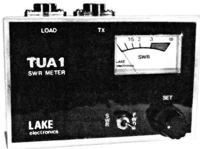
The Lake Electronics TUA1 s.w.r. bridge as built by Tex Swann G1TEX.
