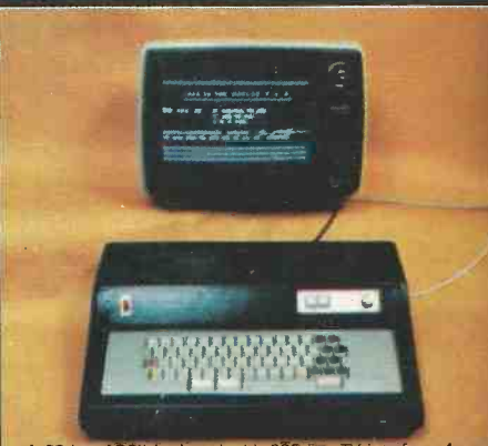
A 63-key ASCII keyboard with 625-line TV interface, 4-page memory and microprocessor interface. Details in our catalogue.
