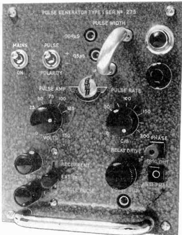
Mercury relay type of pulse generator with rise time of less than 1ns.
