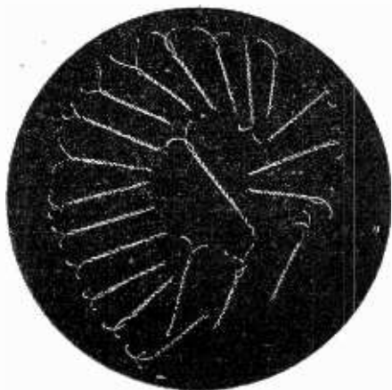
Figs. 7 and 8.—Left, the connecting wires are led through the base and joined to the wave form pattern. Right, printed and etched wave form for use as the stator in the Compton electronic organ. The black portions represent the copper.
