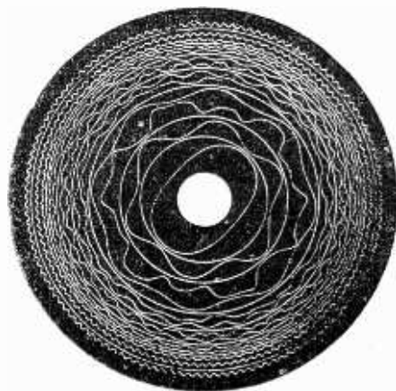
Figs. 7 and 8.—Left, the connecting wires are led through the base and joined to the wave form pattern. Right, printed and etched wave form for use as the stator in the Compton electronic organ. The black portions represent the copper.
