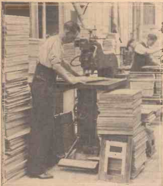
Fig. 1.—A typical Wadkin router, showing work specimens and jig. The cutter runs at the enormous speed of 24,000 revolutions per minute.
