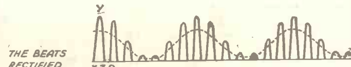
Figs. 9 to 12.—Graphical representation of the working of the first detector valve of a superhet.
