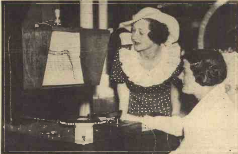
Visitors to the Radio Exhibition were very interested in the H.M.V. tester shown above. The response curve is shown on the screen whilst the pick-up is working. Note the stroboscopic edge to the turntable.
