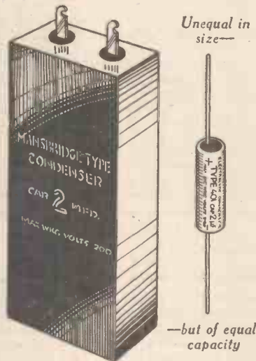
Fig. 2.—A condenser of a few years ago and a similar capacity of the present day. The remarkable saving in space may be gauged from the fact that the two components are drawn to the same scale, and have identical characteristics.
