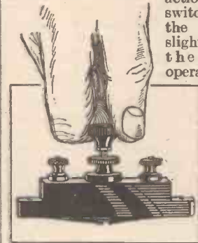
Fig. 9.—A case where one good turn does not deserve another. Screwing a compression condenser down too hard may result in pushing the bottom out.
