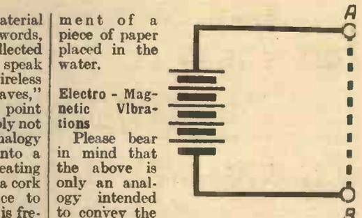
Fig. 2.—There would normally be a voltage or pressure between A and B, but this would vanish if the two terminals were short-circuited as shown by the broken line.
