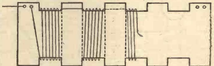
Fig. 3.—Winding a series resistance for a voltmeter.
