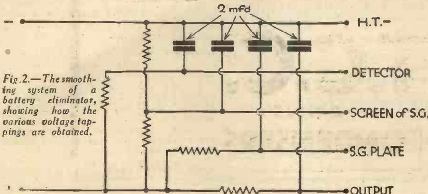
Fig. 2.—The smoothing system of a battery eliminator, showing how the various voltage tapings are obtained.
