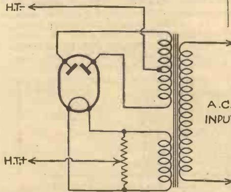
Fig. 1.—A potentiometer used to obtain a centre-tap.
