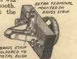
Fig. 10.—How a discarded filament switch may be converted into a 3-point wave-change switch.
