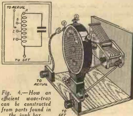
Fig. 4.—How an efficient wave-trap can be constructed from parts found in the junk box.
