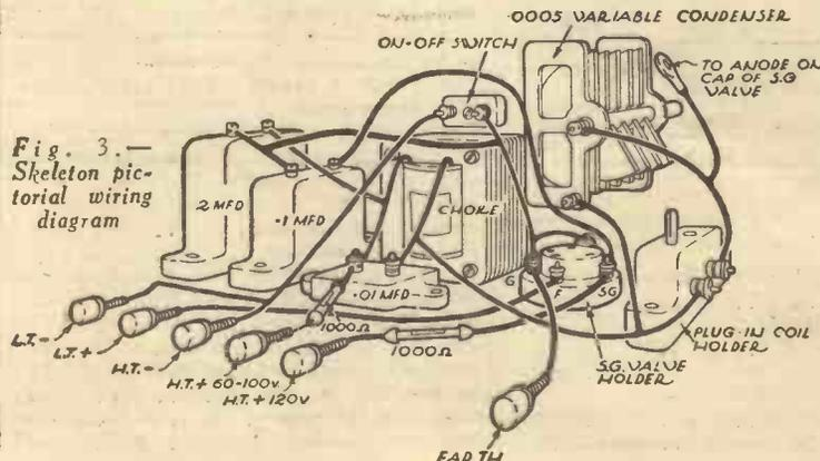
Fig. 3.—Skeleton pictorial wiring diagram
