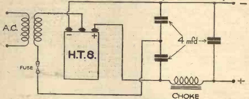
Fig. 1.—The circuit of a mains battery eliminator.
