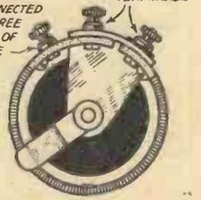
Fig. 5.—How to convert an old filament rheostat into a potentiometer.
