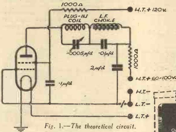
Fig. 1.—The theoretical circuit.
