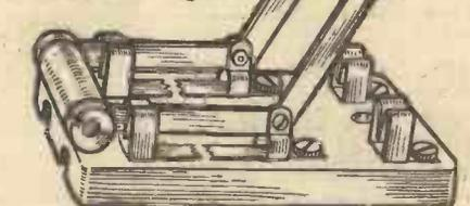
Produced by the Whiteley Electrical, this knife switch is provided with a spark gap, and is very useful for inclusion in the aerial-earth system.
