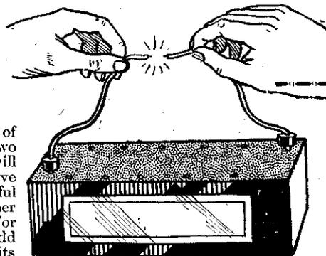
Fig. 3.—Testing the state of a H.T. battery.
