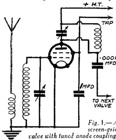
Fig. 1.—A screen-grid valve with tuned anode coupling.
