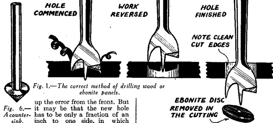
Fig. 1.—The correct method of drilling wood or ebonite panels.
