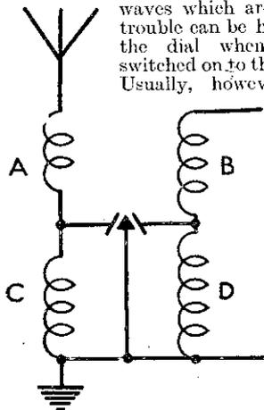
Fig. 1.—Circuit of a dual-range coil with which break-through may occur.
