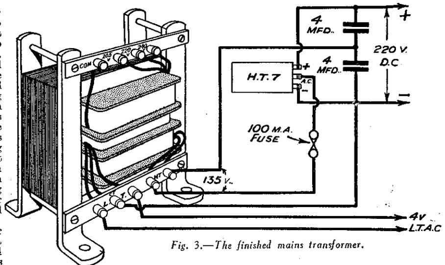
Fig. 3.—The finished mains transformer.
