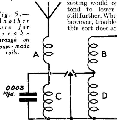
the only cure is to increase the setting of the series aerial condenser and make up for the reduced selectivity by decreasing the coupling between the primary and secondary circuits. If the coil is a home-made one, this can easily be arranged, either by reducing the number of turns in the tapped portion C, in the case of Fig. 4, or by placing the windings C and D farther apart, in the case of Fig. 5.
