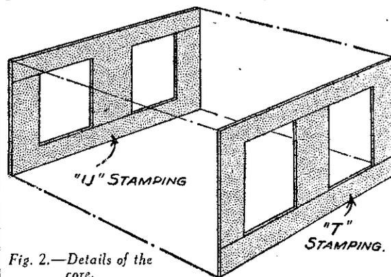
Fig. 2.—Details of the core.
