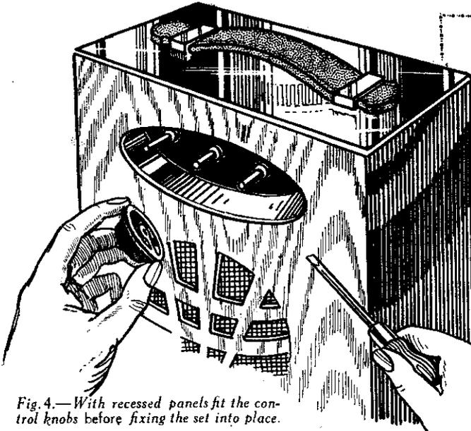
Fig. 4.—With recessed panels fit the control knobs before fixing the set into place.
