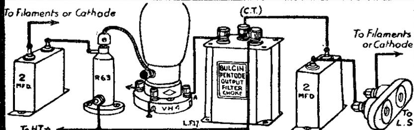
A new L.F. Choke specially designed for use with Pentode valves, electrically centre-tapped to enable a step-down ratio of 2-1 to be obtained. Fitted in new universal mounting case for either chassis (inverted) or baseboard mounting, it is beautifully finished in frosted aluminium with insulated terminals.
