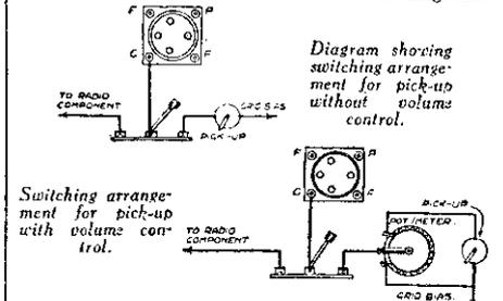
Could you please, therefore, give me a diagrammatic drawing of the switching arrangement for a gramophone pick-up?"—(S. V. T., Hastings).
