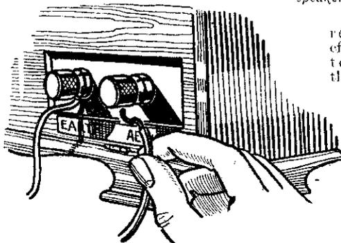
Fig. 9—If crackling noises cease when the aerial is disconnected this is certain proof that they are caused by atmospherics.
