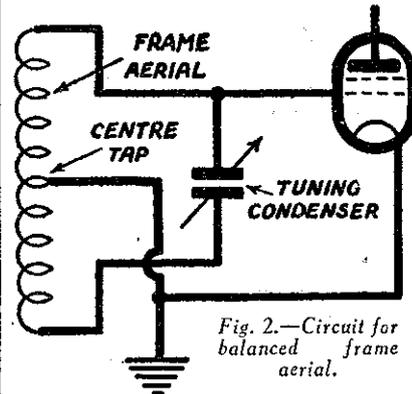
Fig. 2.—Circuit for balanced frame aerial.
