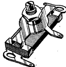
Fig. 7—Suitable potentiometer for eliminating hum.
