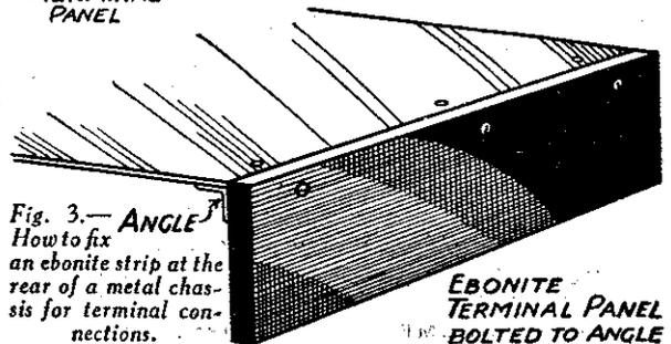
Fig. 3.—How to fix an ebonite strip at the rear of a metal chassis for terminal connections.
