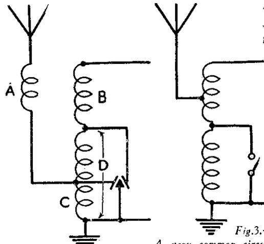
Fig. 2.—Another typical dual-range circuit. Break-through does not occur, but it is unselective on the long waves.
