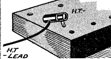
Fig. 3.—The Belling-Lee type of fuse.
