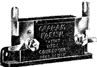
The Graham Farish fixed condenser. These are tested on 750 volts D.C. and are guaranteed accurate to within fine limits.
