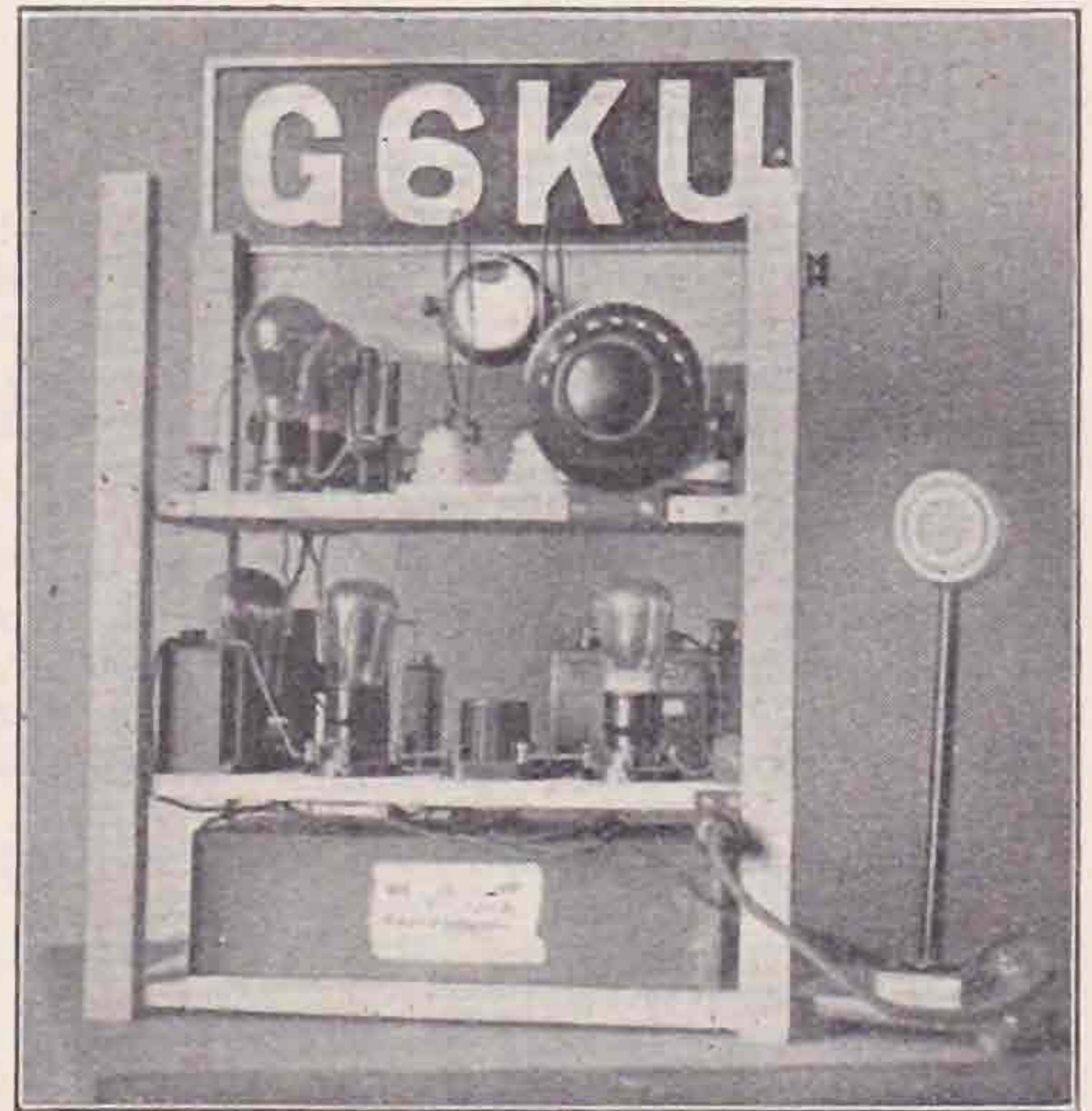
Fig. 4.—Front view of 56 mc. Transmitter and Modulation Panel.
