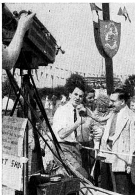
G3CVO (holding the microphone) interviews a visitor in front of the television camera at the "O.B." TV stand at the Dagenham Town Fair, 1952. The camera controls are visible, the operator's hand being on the optical focusing lever, while the box (lower foreground) contains a field telephone for intercom with receiving and monitor site.
