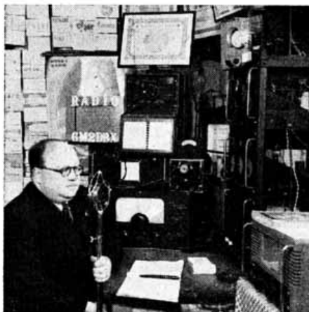
A compact station with a good DX record. At the microphone is Jimmy Taylor (G2MDBX). Equipment pictured includes a workmanlike transmitter, a Commander receiver, and a BC.221 frequency meter.
